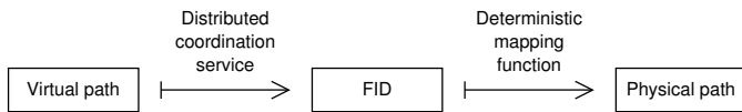
Fig. 2. DUFS mapping from the virtual path to the physical path using File Identifier (FID)
