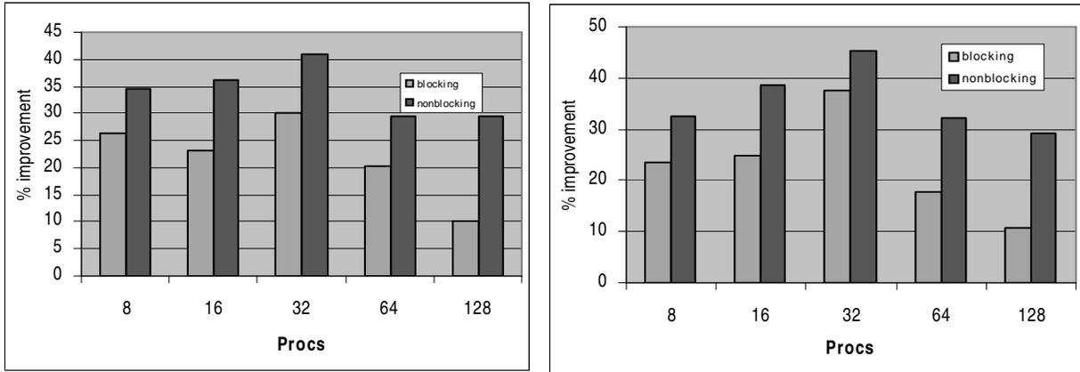
Figure 10: Performance improvement in NAS MG for class B (left) and class C (right)
