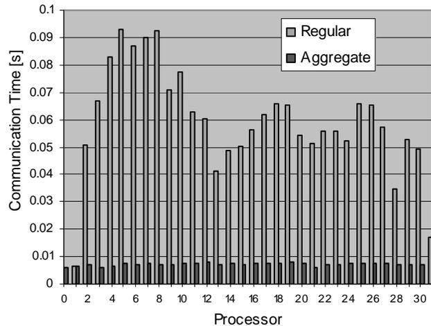
Figure 9: Time spent on communication on each processor in the sparse matrix-vector multiplication in the 32-processor case
