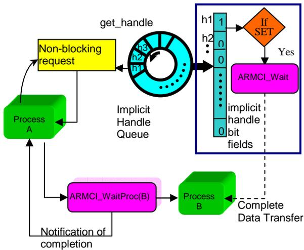
Figure 1: Nonblocking transfer with implicit handle
