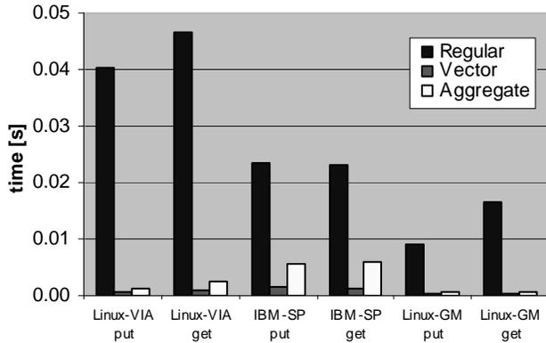
Figure 7: Performance of aggregate, vector, and regular (multiple calls) operations in transfer of 1000 doubles
