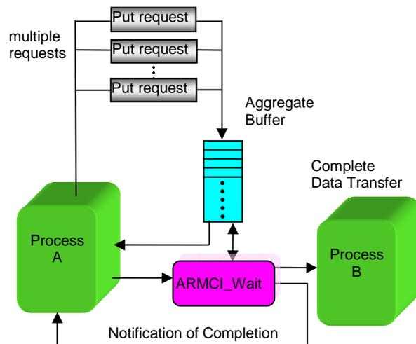
Figure 2: Implicit aggregate data transfer
