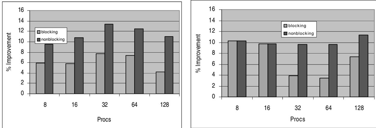
Figure 11: Performance improvement in NAS CG class B (left) and class C (right)
