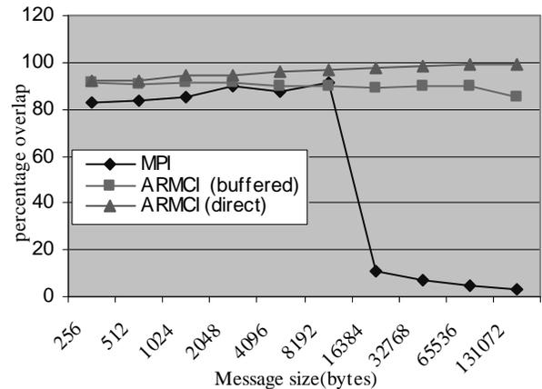
Figure 6: Percentage computation overlap for increasing message sizes for MPI and ARMCI direct and server-based protocols
