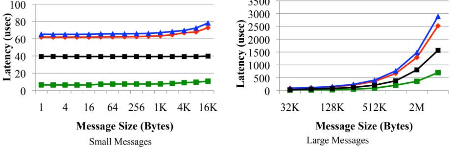
• CUDA IPC significantly improves intra-IOH GPU-GPU communication – 90% improvement for 4Byte and 72% for 4MByte messages
