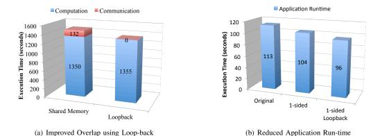
Fig. 3. Performance Improvement in AWP-ODC from Design for Computation-Communication Overlap
