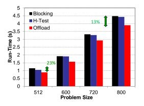
Fig. 4. Run-time comparison of the test\_sine kernel with P3DFFT library
