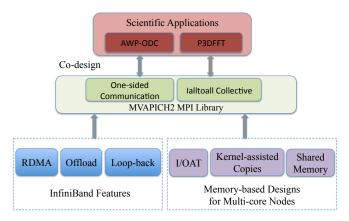
Fig. 1. Co-design Approach for MPI Library, Network and Scientific Applications
