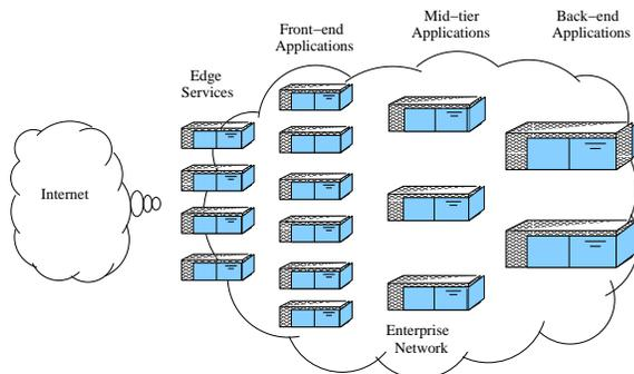
**Figure 1. A Typical Multi-Tier Data-Center (Courtesy CSP Architecture design [40])**
