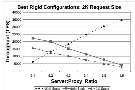
Figure 10. Best Rigid Configurations: Different Average Request Sizes (a) 4KB , (b) 2KB
