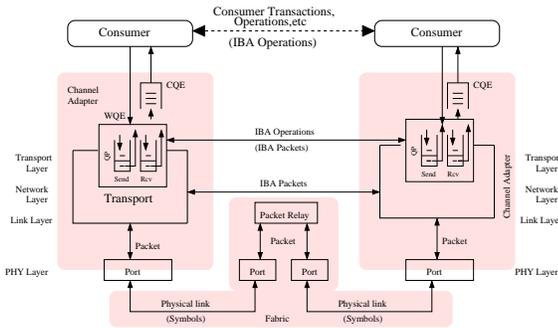
**Figure 2. InfiniBand Architecture (Courtesy InfiniBand Specifications)**
