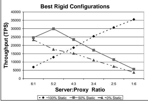
**Figure 8. Best Rigid Configurations: 7-Node Data-Center**
