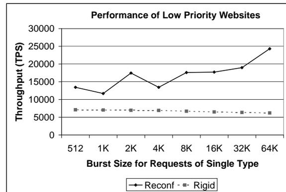
Figure 21. Performance with multiple sites hosted in the data-center: (a) QoS meeting capability for high priority requests, (b) Performance for low priority requests
