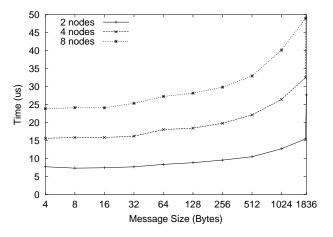
Figure 2. MPI\_Bcast Latency in MVAPICH Using Point-to-Point Communication
