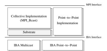
Figure 3. Bridging the Gap between Infini-Band Multicast and MPI\_Bcast
