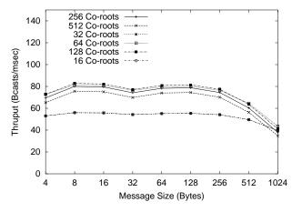
Figure 12. Estimated MPI\_Bcast Throughput for Different Number of Co-Roots (1024 Nodes)
