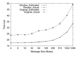
Figure 10. Estimated and Actual MPI\_Bcast Latency (8 Nodes)
