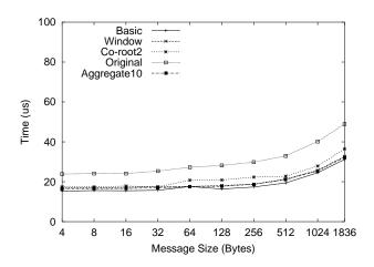
Figure 6. MPI\_Bcast Latency for Small Messages Using Various Multicast Schemes(8 Nodes)
