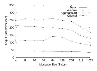
Figure 8. MPI\_Bcast Throughput (8 Nodes)
