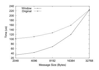
Figure 7. MPI\_Bcast Latency for Large Messages (8 Nodes)
