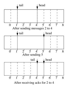
Figure 4. Sliding Window Buffer Management
