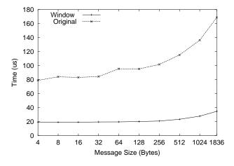
Figure 11. Estimated MPI\_Bcast Latency for Small Messages (1024 Nodes)
