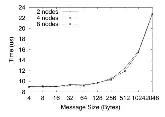
Figure 1. InfiniBand Multicast Performance
