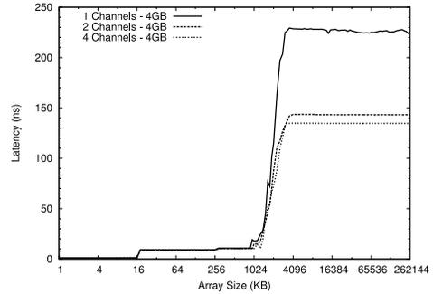
Figure 1. Main Memory Access Latency with Varying Numbers of Channels
