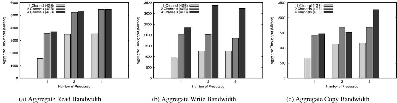
Figure 2. Bensley Memory Throughput for Varying Numbers of Channels
