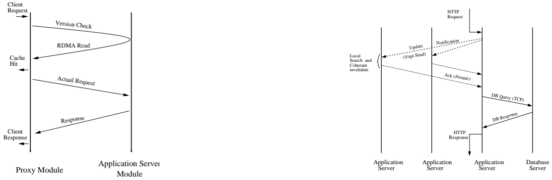
Figure 6: Design for (a) RDMA based Strong Cache Coherence Validation and (b) Coherent Invalidation
